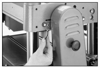
Figure 24. Feed roller height adjustment.
